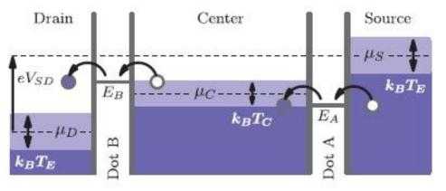
Resonant levels provide contacts with conductance
